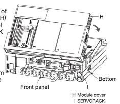
8. Fix the module cover to the SERVOPACK Retention clip angle by pushing in the end protrusion retention clips on the left and right side of Push the clips in the the module cover, while directing their by the arrow so the clip will go into the SERVOPACK. angled end protrusions to enter the SERVOPACK. Retention clip Retention clip
